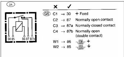
So how do I hook up the new cube-shaped relay? The bottom of the relay (3A) is shown with the modern as well as the old terminal designations. You will need to refer to the wiring diagram for your vehicle to determine which color wire goes where.
