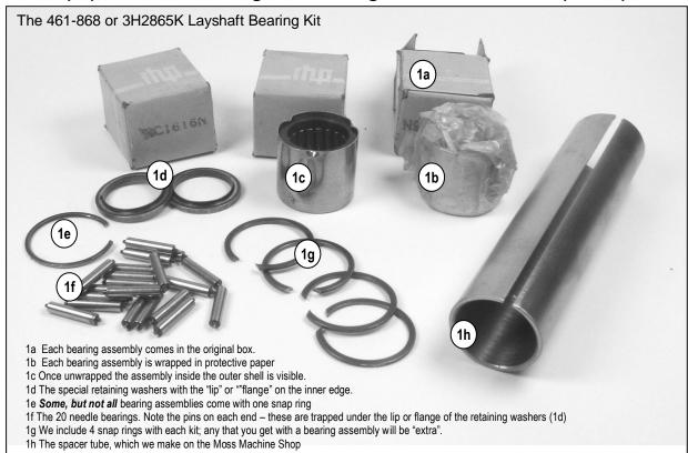
We suggest you leave the bearing assembly (1c) alone until you have read the rest of this... the bearing assembly is a lot easier to deal with as a unit than as 20+ separate bits.
