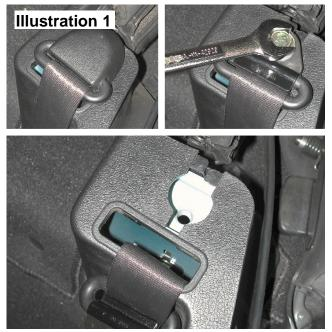
**2.** Install the lower spacers on both sides of the car per drawing:
