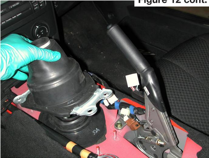
13. Pull up around the circumference of the lower shift boot to dislodge it from the transmission tunnel. Then pull it off of the shifter. Figure 13.
