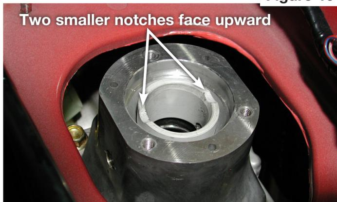
20. Take the shifter assembly and gently guide it straight down into the transmission. The plastic bushing on end of the shifter should slide easily into the cup in the shift turret and the shifter ball should rest on top of the plastic bushing you installed. Next guide the shift spacer adapter over the top and ensure the set screws line up with the slots in the shifter pivot ball. Figure 20.
