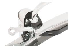
The badge bar has a boss attached to the fixing brackets which should allow the tightening of the bolts holding the overrider so that the badge bar is held firm. If a spot/fog lamp bracket is not used, you may need to use some packing washers to help fill the void.
