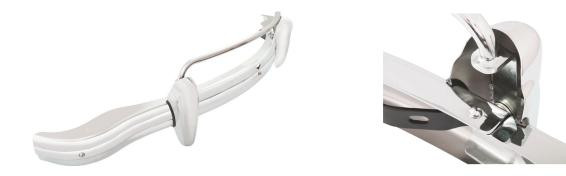
The badge bar can fitted with or without the optional factory option spot/fog lamp brackets as these are also fitted in the void between the bumper face and overrider but attach direct to the bumper.
