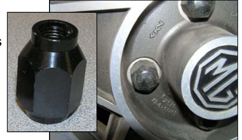
Kelvin Dodd's original LE wheels and wheel nuts. New 264-990 or BHH 2269 nut on left.
