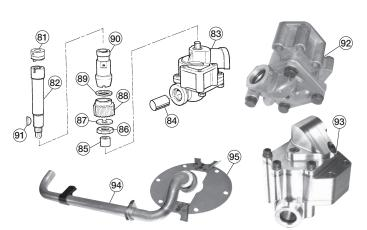
Internal Engine Six-Cylinder, Oil Pump
