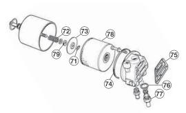
Oil Filter Housing, Series II From (e) 7R.2298 (FHC & OTS) and 7R.35583 (2+2)
