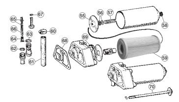
Oil Filter Housing, 3.8lt, Series I 4.2lt, Series II to (e) 7R.2297 (FHC & OTS) & 7R.35582 (2+2)
