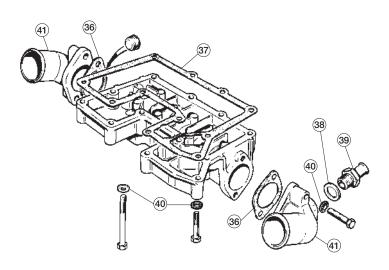
External Engine V12, Oil Cooler
