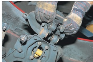
The shock absorber is still retaining the spring. Next, the steering knuckle can be folded out of the way.
