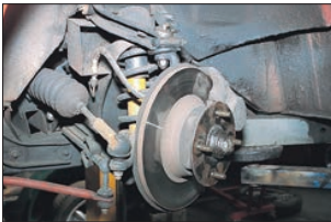
A typical example: the TR6 has two wishbones on each side.
