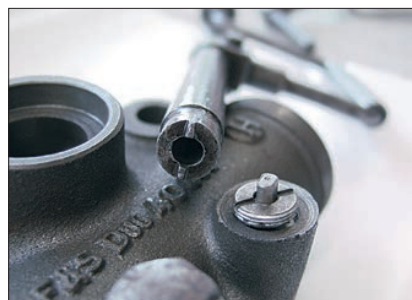
... can only be unscrewed with a special tool (which can, however, be easily fabricated).
