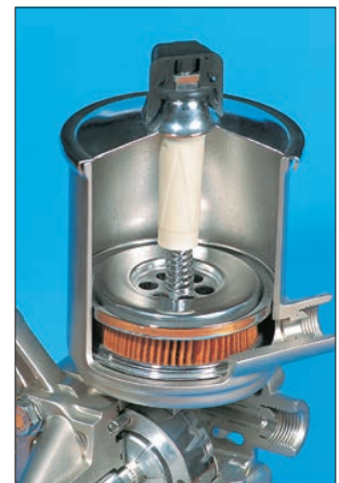
The filter in the fluid reservoir provides protection against dirt.
