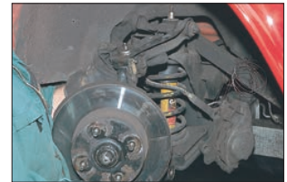
The steering knuckle can now be removed, together with the wishbone.
