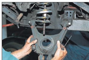
... the camber adjustment plates, can be removed with the help of a spring compressor.
