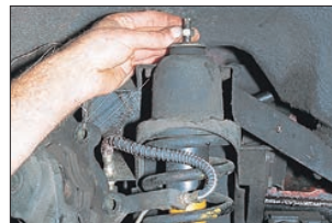
... the upper mounting bolt can be undone without danger.
