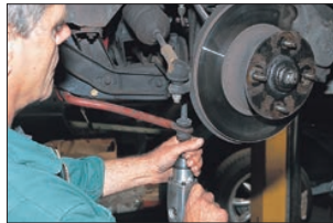
Dismantling starts with the anti-roll bar attachment.
