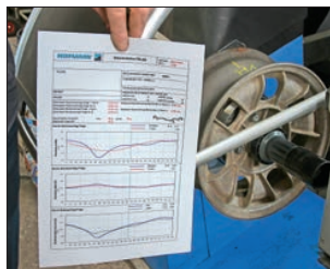
The inspection sheet provides a good deal of information: here it shows the presence of impacts to the top and side of the rim. The bead seat, on the other hand, is unremarkable.
