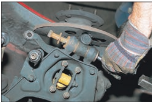
The lower retaining bolt can be withdrawn safely.
