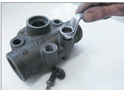
Control valves: after the sealing caps have been taken apart, the valves ...
