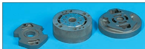
The shape of the contour ring in the rotational group is reminiscent of a Wankel engine. The centrifugal force pushes the rotor vanes to the outer edges and the fluid flows under pressure through the side plates.
