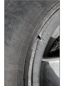
These wheels have had it: the fracture (on the left) has occurred as the result of attempts to repair the wheel. In the photograph in the middle, the distortion has gone too far down into the rim well; on the right, the damaged area is too large.
