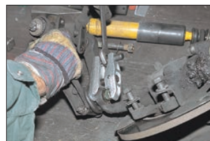
On the workbench: the lower wishbone link needs to come out.
