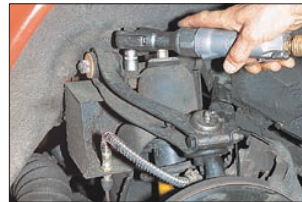
The upper wishbone is not held under tension.
