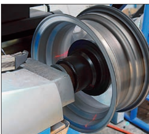
The final doubts are dispelled: the laser measurement reveals any impacts to the top or side of the rim.
