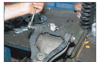
Then the bracket on the upper wishbone can be undone.
