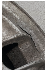
These wheels have had it: the fracture (on the left) has occurred as the result of attempts to repair the wheel. In the photograph in the middle, the distortion has gone too far down into the rim well; on the right, the damaged area is too large.
