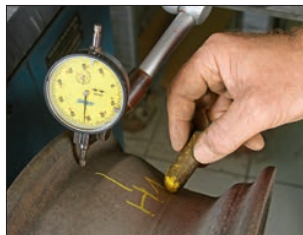
On the inside of the rim, the specialist determines and marks the highest point of the imbalance.
