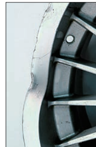
These wheels have had it: the fracture (on the left) has occurred as the result of attempts to repair the wheel. In the photograph in the middle, the distortion has gone too far down into the rim well; on the right, the damaged area is too large.
