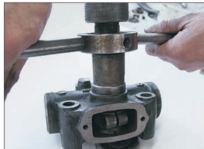
... the screw, a puller can now be used to extract the rod and remove the piston lever.
