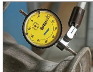
The rim flange is also checked. Any small chips here can lead over time to the development of cracks.
