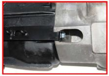
*Note:* When the gearbox is bolted in situ you can then fit the retaining bush to the side-relay bracket and attach the original clutch lever mechanism to the new side-relay bracket as you would on the original gearbox. See point 17
